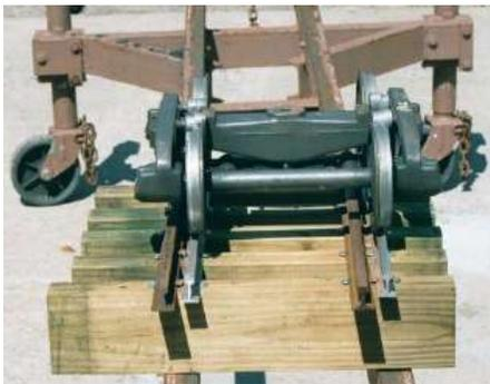
One of the trucks was placed on the segment of aluminum rails, with the flanges touching one side rail.
