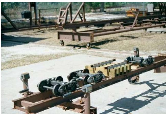
LCRR made available three types of rail truck in the same scale; the differences were in the materials of the wheels. They were: cast iron in new condition; cast iron in worn condition; and steel in new condition.
